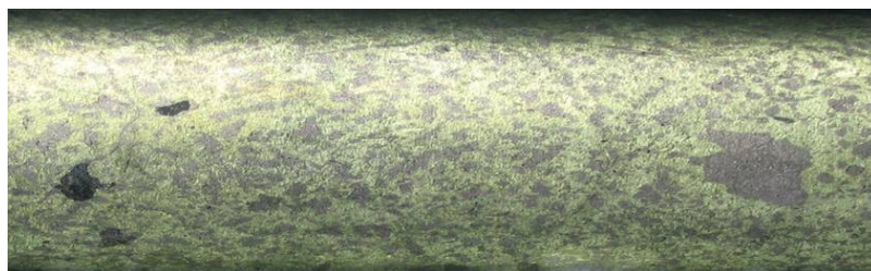
Drill core from END 04 – chalcopyrite rich massive sulphide
